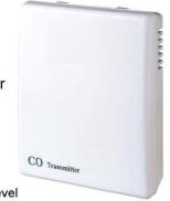
BCT3100-CO series is specifically designed to detect and transmit carbon monoxide level in the enclosed or semi-enclosed car parks and to regulate the environment according to the measurement of carbon monoxide. It is designed for easy installation and minimum maintenance during operation. RS-485 communication interface is available as an option with independent address, thus it can be connected with a PC or DDC/PLC.
