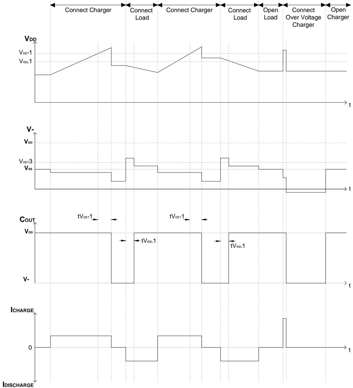
3. Overdischarge, Discharging Overcurrent and Short operations
