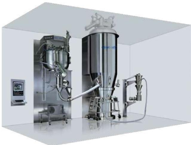
Freund-Vector's horizontal granulation suites can be executed with both top & bottom drive systems and installed within single or adjacent processing rooms. The equipment layout is based on a through-the-wall design to minimize processing space and simplify cleaning the equipment.
