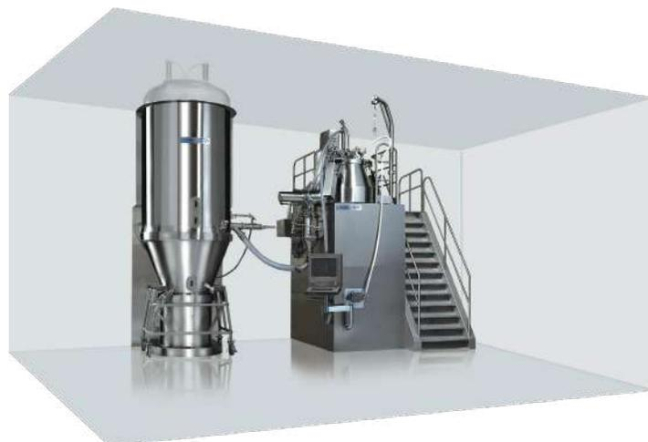
Freund-Vector's vertical granulation suites can be installed on several floors of a pharmaceutical facility. Gravity is utilized to provide a more efficient flow of product.
